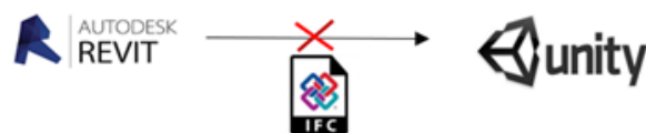
Figure 3: The * .ifc file format system modeled with Autodesk Revit in the BIM platform cannot be detected by the Unity UI because of interoperability problem.
