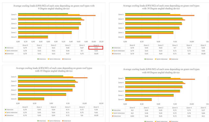
Figure 4: Average cooling loads of each zones depending on green roof types and angle of shading devices.
