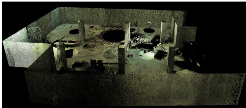
Figure 4: Bahariye station laser scanning model.
