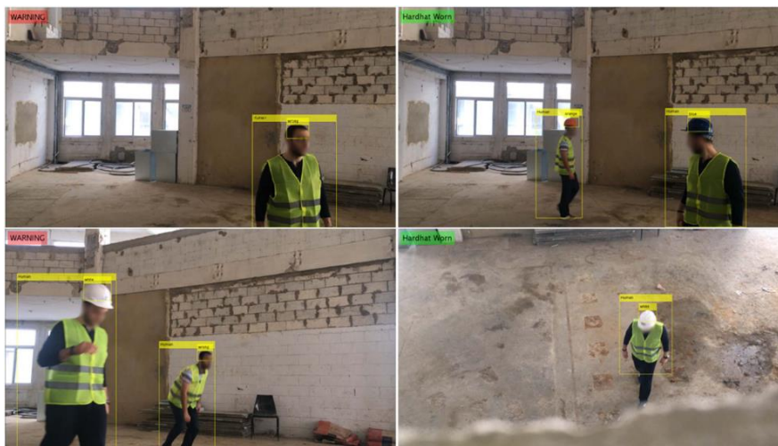
Figure 6: Test examples from hardhat detection (Mnemyneh et al., 2019).
