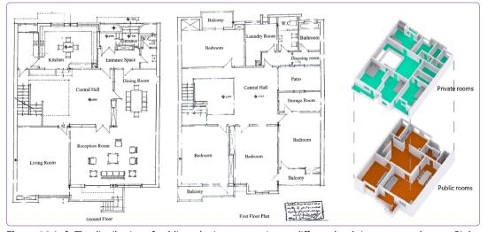
**Figure 14.** Left: The distribution of public and private rooms in two different levels in two-storey houses. Right: The ground floor is generally dedicated to the public spaces while the upper floor features private rooms.
