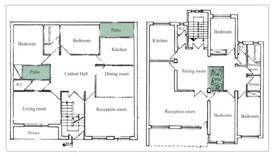
Figure 11. The patio is used to illuminate the inner spaces deprived of natural light.
