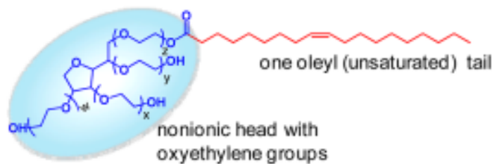
Figure 1.9: The molecular structure of Tween 80, blue part denotes hydrophilic head and red part denotes hydrophobic tail (Athas et al., 2014)
