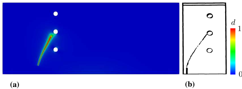
Figure 2.19: Crack trajectory of the asymmetric notched three point bending test obtained by (a) the current work, and (b) the experimental work by Bittencourt et al. [96]
