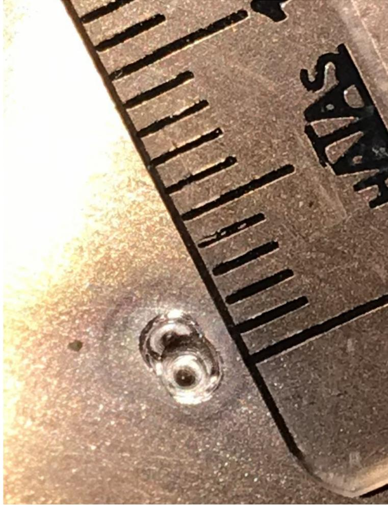
Figure 6.9: Photo of copper table after test. The beam size is measured as 2mm
