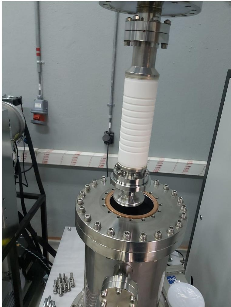
Figure 6.5: Photo of ceramic structure and focusing electrode placement
