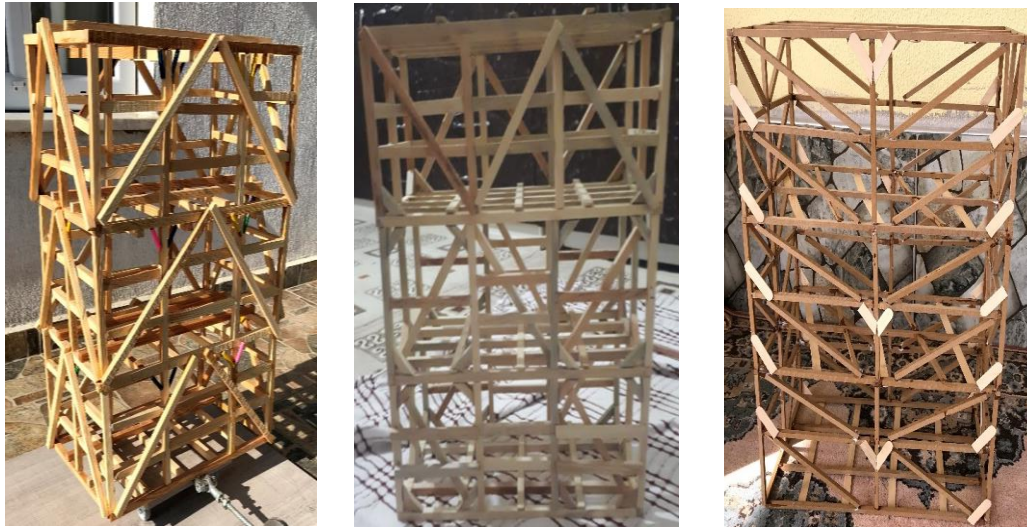
Figure 4.22. Some students' earthquake resistant wooden building products
