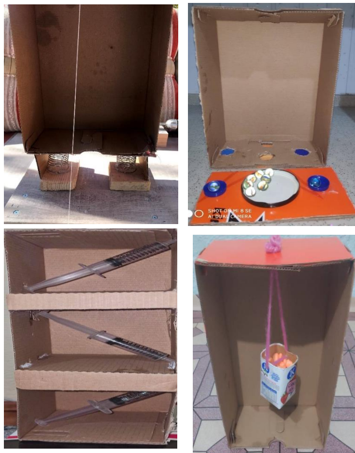
Figure 4.29. Examples of the students' products with the base isolation, the seismic damper and the tuned mass damper technologies
