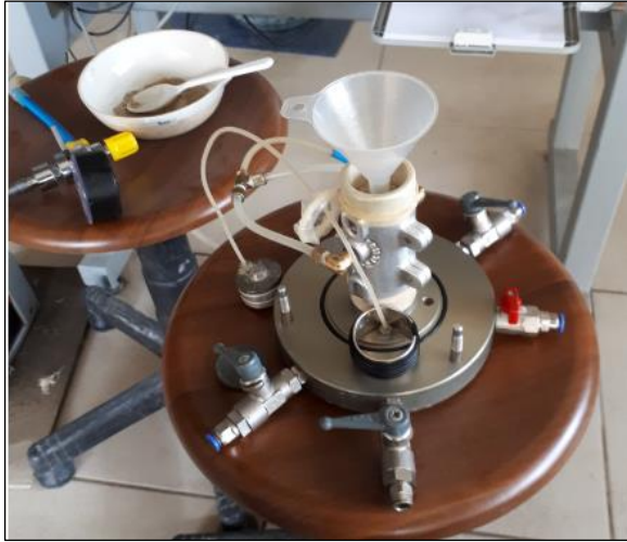
Figure 3.5. Tapped funnel deposition method
