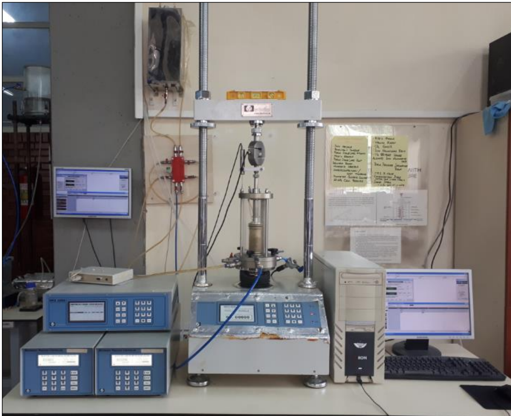
Figure 3.3. VJ TECH automated triaxial test system
