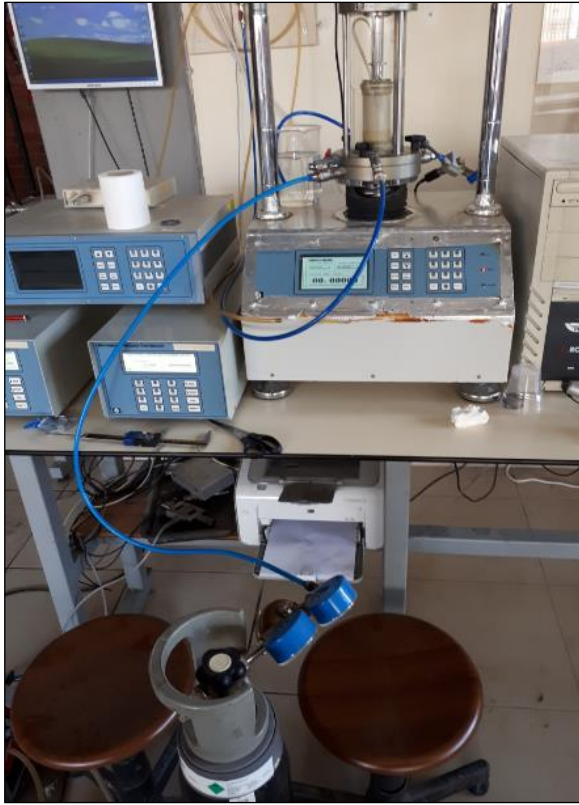
Figure 3.8. Passing CO 2 through the sample
