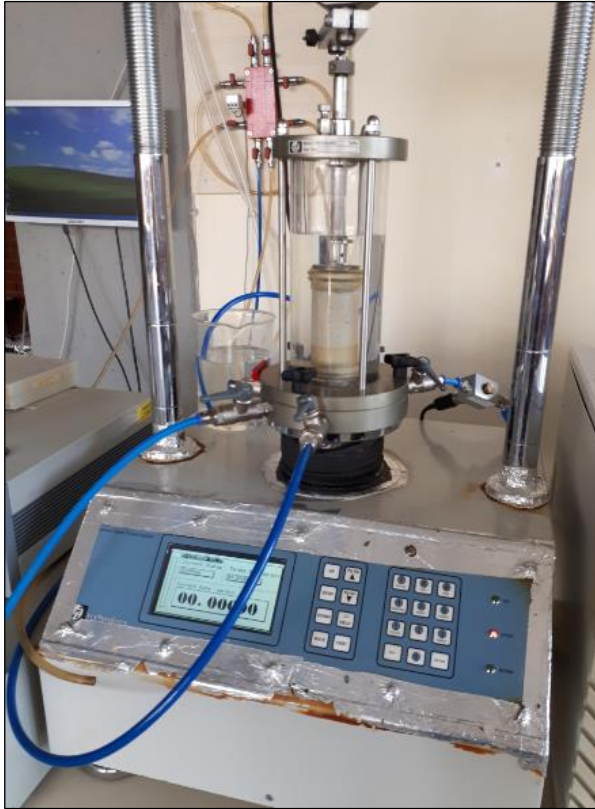
Figure 3.7. Filling the cell with water
