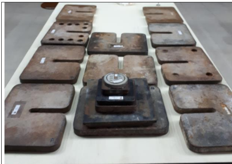
Figure 3.13. Weights used for oedometer tests
