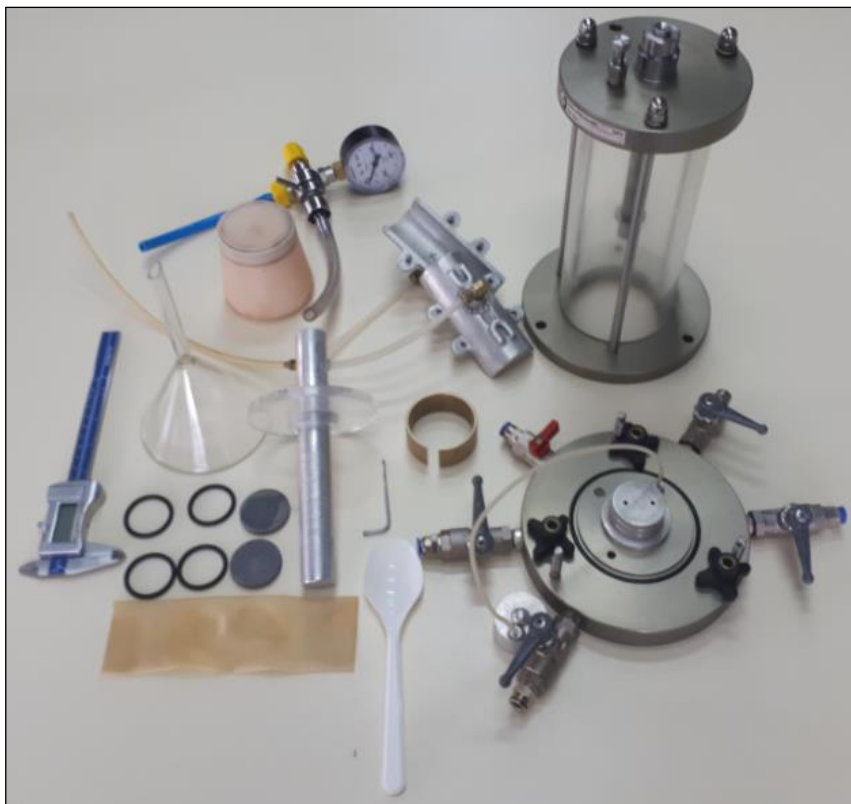
Figure 3.4. Apparatus used in triaxial tests
