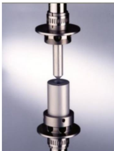
Figure 3-7. Liquid test apparatus for DMA (Metravib, n.d.)
