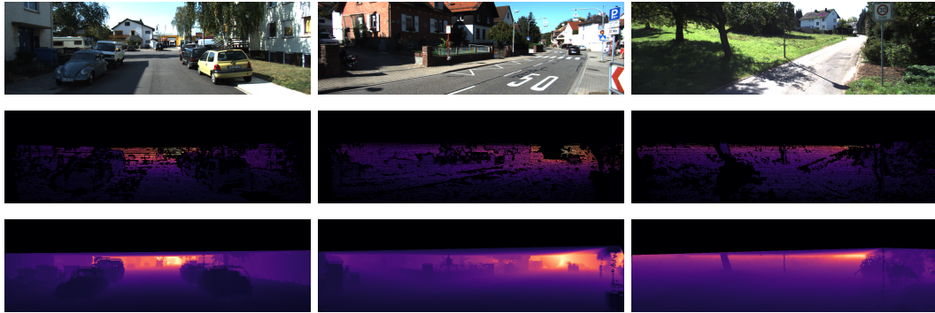
Figure 2.23: KITTI Dataset [22] sample images. From top to bottom: Sample Image, Sparse Ground Truth Depth Map, Dense Ground Truth Depth Map
