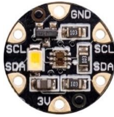
Figure 4.2 The color sensor used in Light Order game materials
