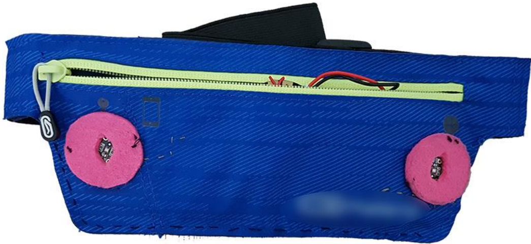
Figure 4.21 Interactive belt v1 (The sensors were framed but not covered)
