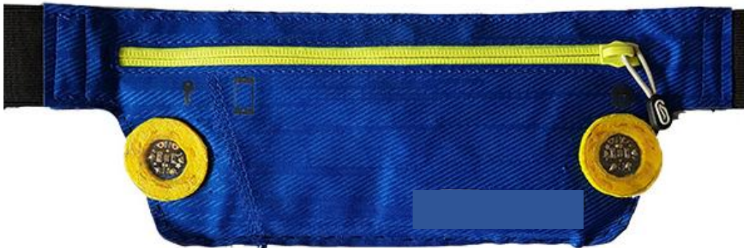
Figure 4.22 Interactive belt v2 (Sensors were framed and covered)
