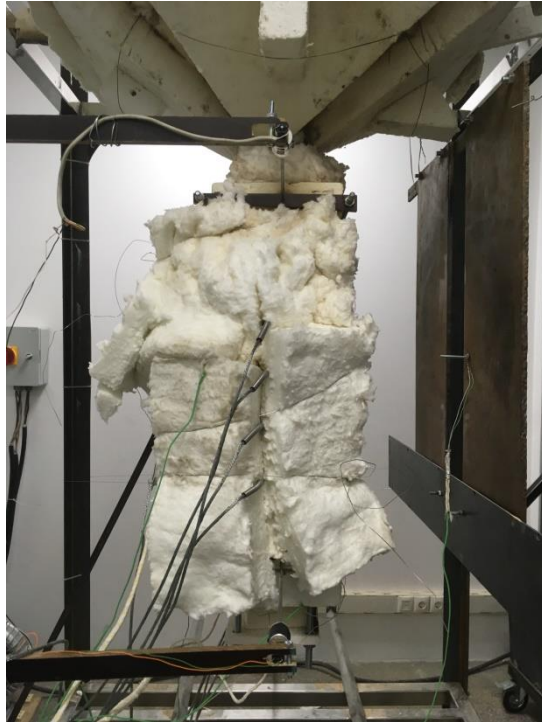
Figure 6.19. Test section, well-insulated on three sides with ceramic insulation.
