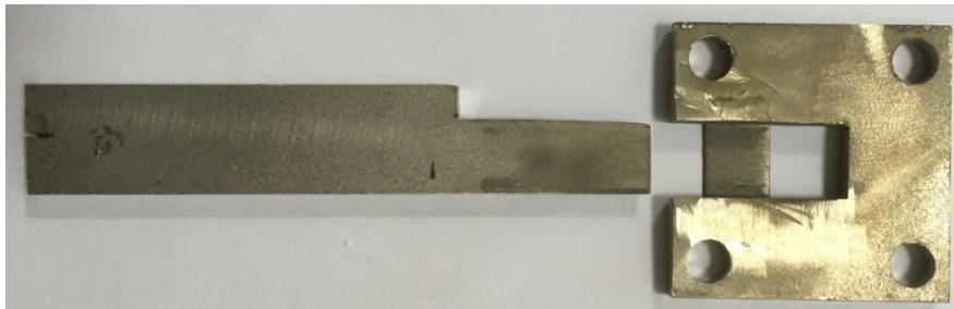
Figure 6.6. Shutoff valve used to stop the particle flow.
