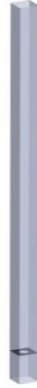
Figure 7.1. Square tube test section and orifice plate used in modeling the experimental setup.
