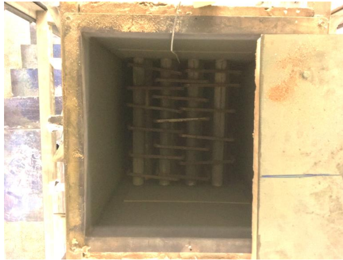
Figure 6.20. Top view of the hopper, where U-shaped steel rods are placed over the heating tubes to promote conduction inside the hopper and reduce temperature gradients.
