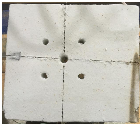
Figure 6.8. Inlet temperature measurement block with grooves cut for thermocouples wires.
