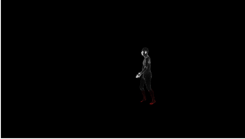
Figure 5.3: Occluded (red) and visible (white) vertices of the frame given in Figure 4.4 (b) as the output of the step 1 of Algorithm 4
