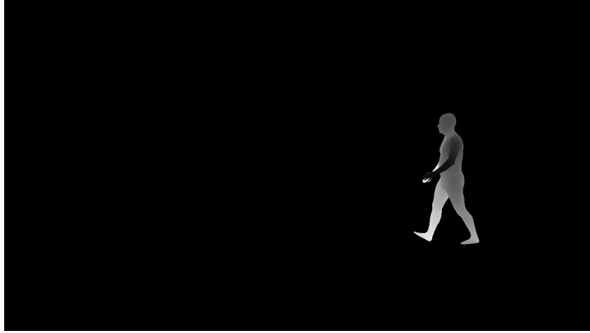
Figure 5.2: An example depth image of an SMPL body. Only the depth information of the SMPL body exists. The closest point to the camera is shown with black while the farthest point is shown with white.
