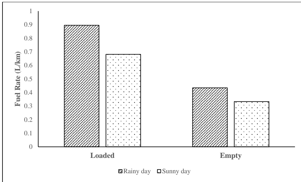
Figure 4.7. Fuel Rates for Loaded and Empty Trucks in Rainy and Sunny Days
