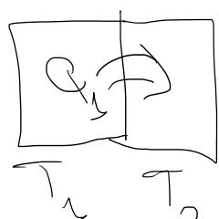
$$\Delta S = -\frac{Q_1}{T_1} + \frac{Q_1}{T_2} = Q_1 \left( \frac{1}{T_2} - \frac{1}{T_1} \right)$$
