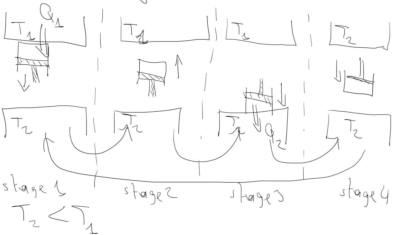
$T V^{2/3} = \text{const}$  on an adiabatic curve
