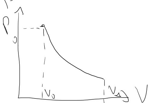
$$W = \int_{V_0}^{V_1} P dV = NkT \int_{V_0}^{V_1} \frac{dV}{V}$$
