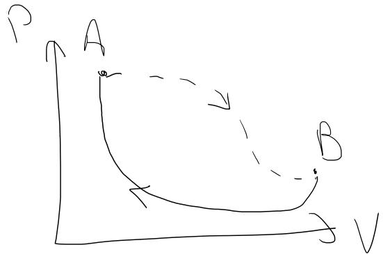
$$\Delta S = \int_{(irr)} \frac{dQ}{T} + \int_{(rev)} \frac{dQ}{T} \geq 0$$
