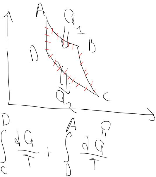
$$\oint \frac{dQ}{T} = \int_D \frac{dQ}{T} + \int_B \frac{dQ}{T} + \int_C \frac{dQ}{T} + \int_D \frac{dQ}{T} + \int_A \frac{dQ}{T} + \int_B \frac{dQ}{T} = 0$$
