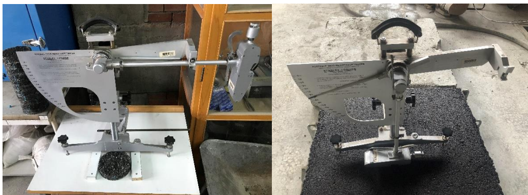
Figure 3-9, left: BPN measurement on disk specimen, right: BPN measurement of asphalt block
