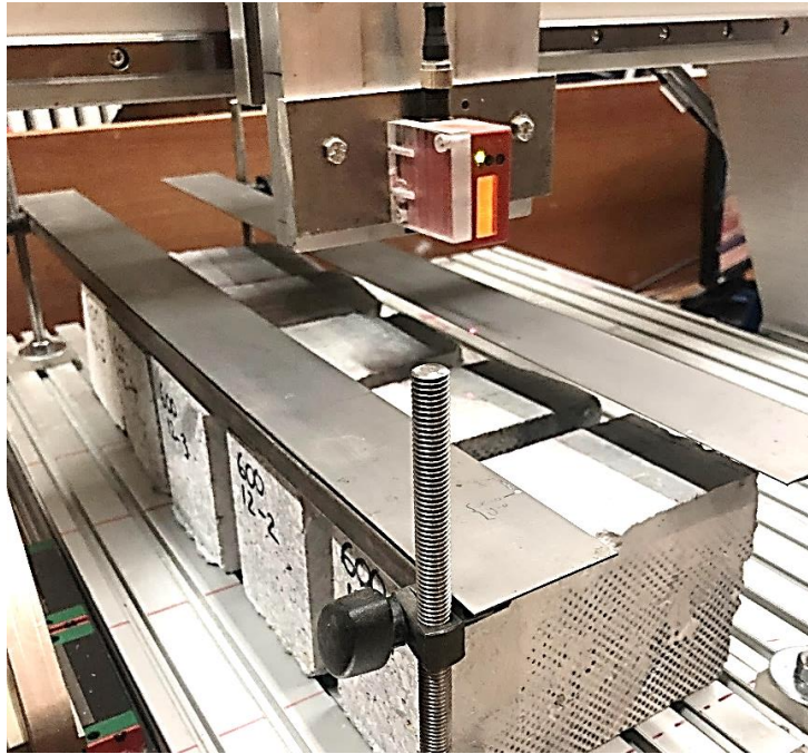
Figure 3-2, Close up of guide frame and samples under scan
