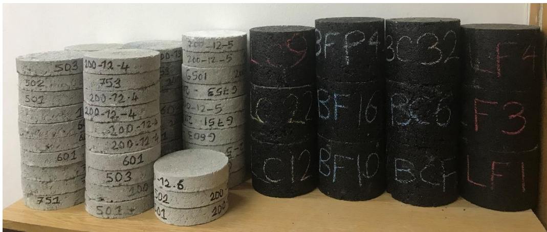
Figure 3-7, Concrete and asphalt samples compacted with SGC
