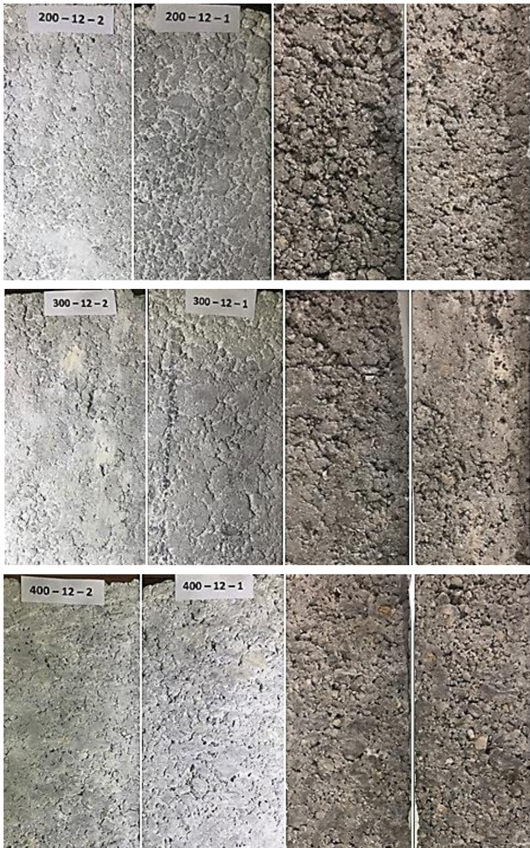
Figure 6-4, RCCP samples with 12 mm stone, before (two pictures on the left) and after 50 cycles of freeze-thaw (two pictures on the right)
