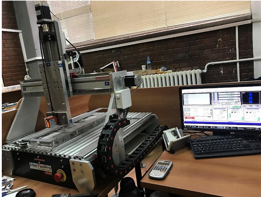
Figure 3-1, The developed Non-contact 3D scanner
