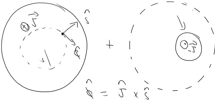
$$\begin{aligned} \vec{B}(\vec{s}) &= \frac{1}{2c} \vec{J} \times \left( \frac{\vec{r}}{r} - \frac{\vec{s}}{s} \right) \\ &+ \frac{1}{2c} (-\vec{J}) \times \left( \frac{\vec{r}}{r} - \frac{\vec{s}}{s} \right) \\ &= \frac{1}{2c} \vec{J} \times \left( \frac{\vec{s}_2}{s_2} - \frac{\vec{s}_1}{s_1} \right) \end{aligned}$$
