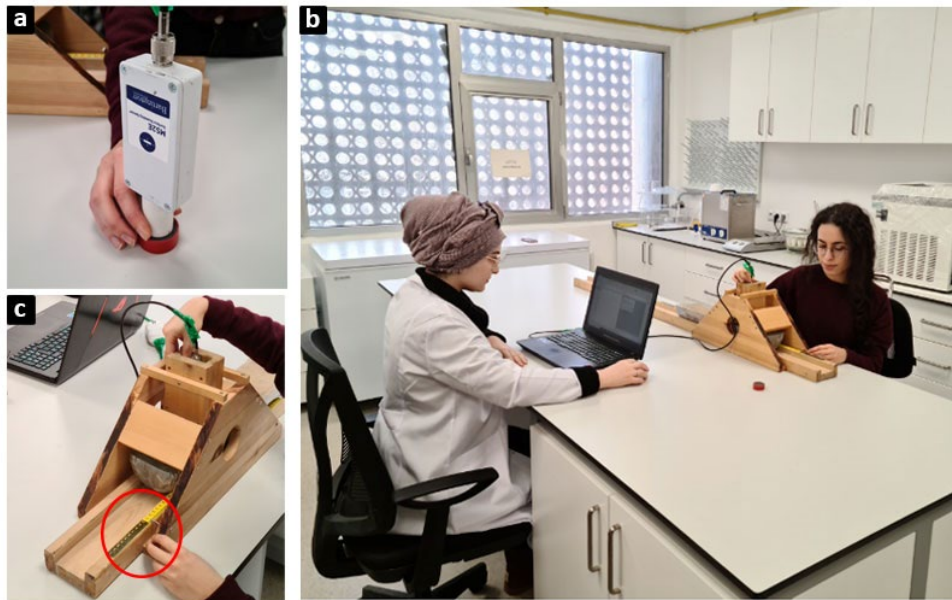
Figure 3.9. Magnetic susceptibility measurement in sediment cores using the Bartington MS2E surface sensor. a) Calibration process repeated for each core before starting the measurement. b) Magnetic susceptibility measurement by one end of the sensor attached to the computer and the other end touching the sediment surface. c) Triangular-shaped wooden apparatus that ensures proper contact of the sensor with the sediment. The nail indicating the measured level is indicated with a red circle.
