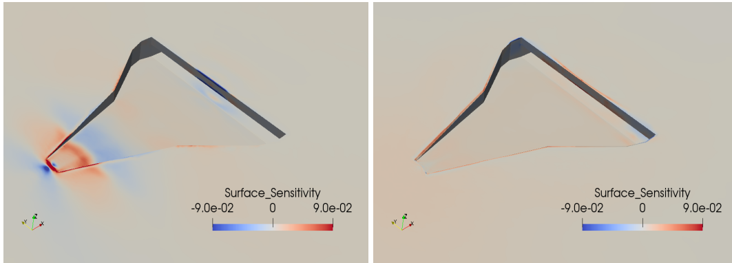
Figure 4.2: Lift calculated surface sensitivity; Left: Baseline; Right: Optimum design.
