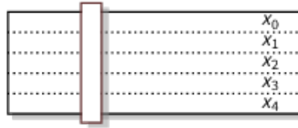
Figure 3.3: Substitution layer of Ascon. Figure was taken from the cipher's official website https://ascon.iaink.tugraz.at/images/state_vertical_small.png
