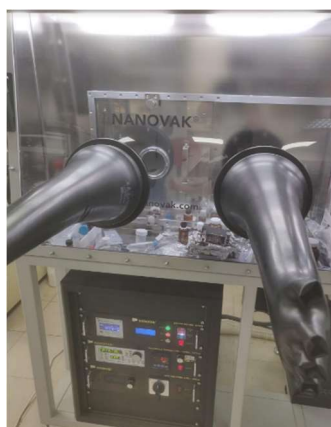
Figure 4.4 Nanovak thermal evaporator located inside the glovebox.
