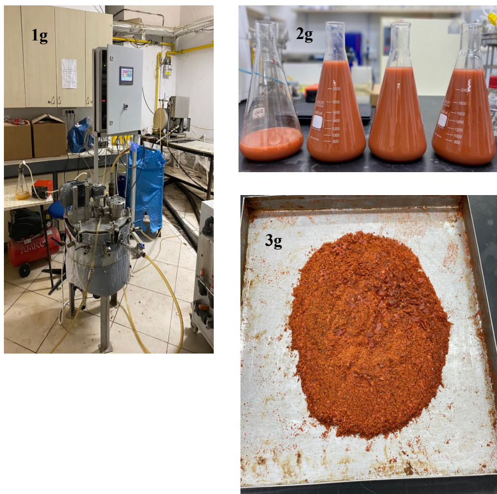
Figure G.1. Pictures of the 10 L scale up experiment. 1g: 30 L industrial type fermentor with 10 L fermentation medium, 2g: Post-fermentation view of D medium prior to cell collecting, 3g: Total biomass collected from 10 L fermentation medium.
