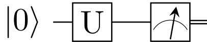
Figure 3.2: A single qubit circuit representation. The qubit starts with the |0\rangle initial state. A unitary operation U is applied as shown with the box. Then, the measurement operation is performed as shown with a meter sign in a box.
