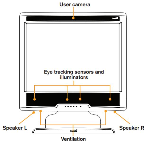
Figure 4: Front display of Tobii T120 eye tracker
