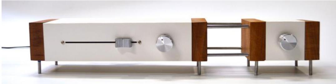
Figure 2.13 - In resemblance to a retro music set, OLO has no screen for enabling interaction unlike the modern music-playing artefacts; instead, it carries a slider and two dials for navigation through time and control of the music's volume, which is the purpose thereof (Odom & Duel, 2018).
