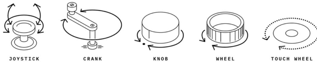
Figure 6.9 - Components appropriate for input through circular motion.
