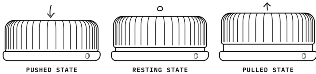
Figure 6.28 - Lateral view visualising the pushed and pulled states of the wheel, both of which spring back to the resting state for enabling repetitive input for furthering the tolerance input. In addition, a widened base for supporting the grasp of the hand that anchors the base.
