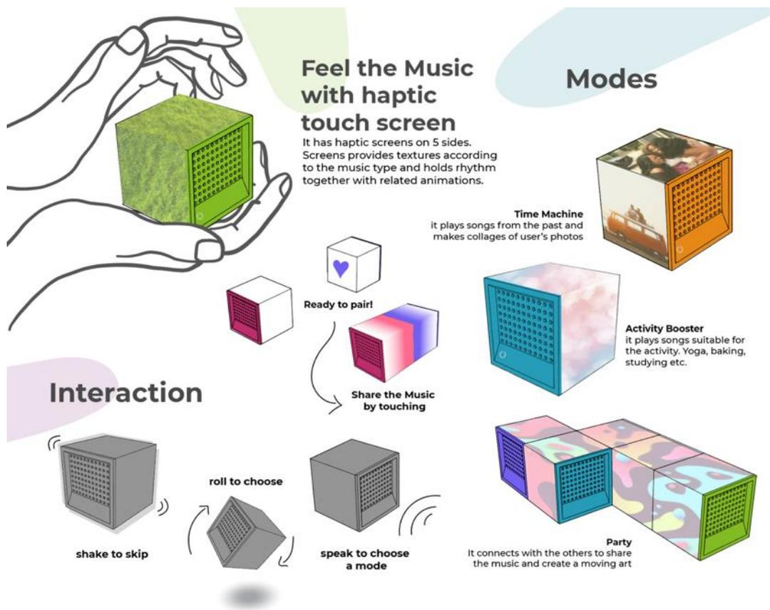
Figure 4.16 - P1's Dream Cube, which augments the music-listening experience through multisensorial media enhancements such as tactual and visual feedback: relying on tangible interactions as the control scheme.
