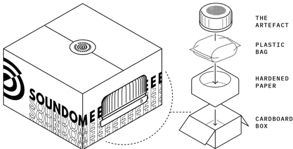
Figure 6.37 - Outer packaging element (left) and the nesting of all elements (right).
