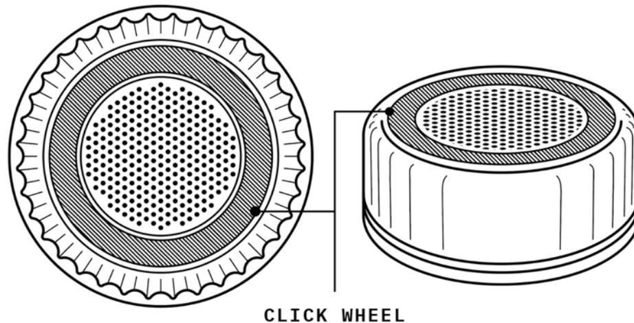
Figure 6.31 - The click wheel encircling the screen is used for adjusting secondary controls that don't have effect on directionality, temporality, and tolerance of music playback.
