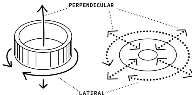
Figure 6.15 - Motion perpendicular to the lateral movement on a wheel.
