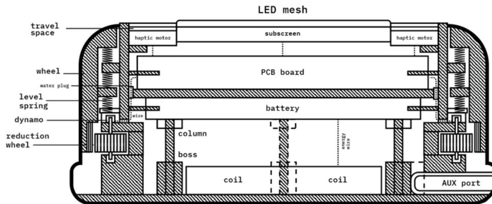
Figure 6.33 - An approximate drawing as a proof of concept that the enclosed space is adequately spacious for constituting the functions, features, and qualities in question.
