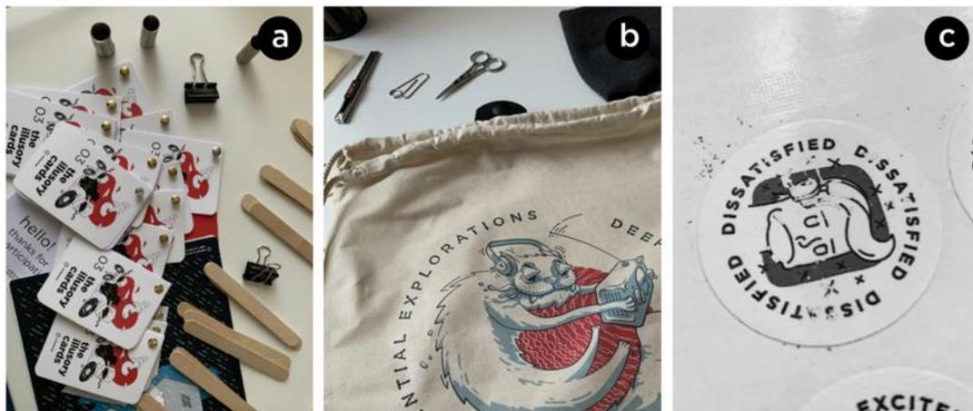
Figure 4.7 - Several photos from the manufacturing process: insertion of rivets into ‘The Illusory Cards’ and cutting the springs into keyrings for ‘Veiled Listening Session’ activities (a), testing the properties of the cloth bag and how it holds the research material (b), a close-up from the defective (peeling) batch of stickers that failed to adhere onto polypropylene base which then was corrected (c).
