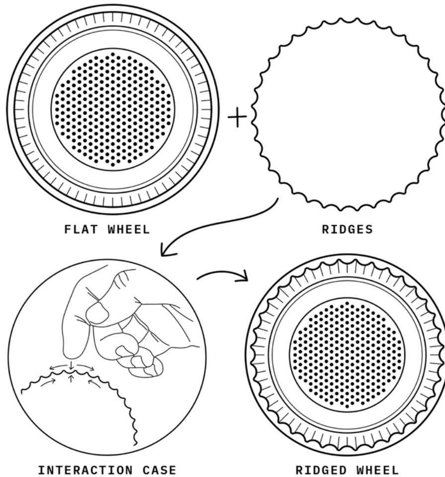
Figure 6.29 - Visualising the inclusion of ridges onto the wheel for supporting the omnidirectional rotation atop the user's fingers – *no, the ridges don't represent serrations.*
