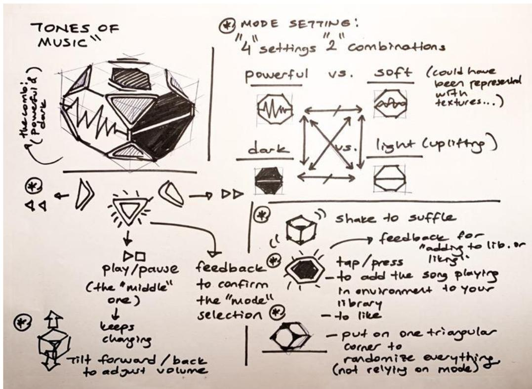
Figure 4.24 - The main faces were broken between dichotomies located at two opposing faces: *Soft* and *Intense*, *Light* and *Dark*, and two randomisation faces for shuffling. Furthermore, the cut-off corners work like an extension of traditional music-player controllers for starting, stopping, and winding forward the music pieces, while also enabling randomisation if it stands on a corner after rolling.
