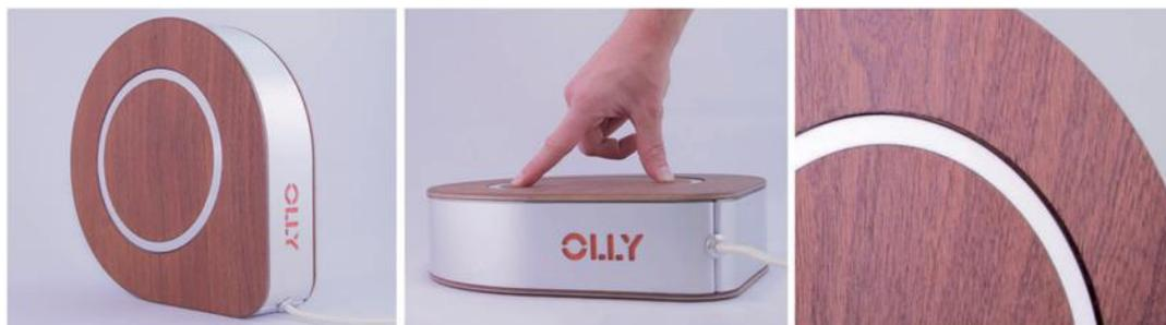
Figure 2.14 - Physical form, interactivity, and material qualities of Olly, respectfully in order. Navigation between the tracks is done through the rotation of its hand-sized dial (Odom et al., 2019).
