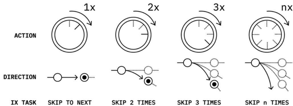
Figure 6.10 - Interaction between user and wheel can be represented like this: highlighting how action, direction, and interaction task correlates to each other.
