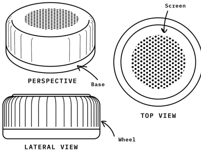
Figure 6.26 - Perspective, lateral, and top/bottom views of the Artefact with the inclusion of a base, wheel, and a placeholder display.
