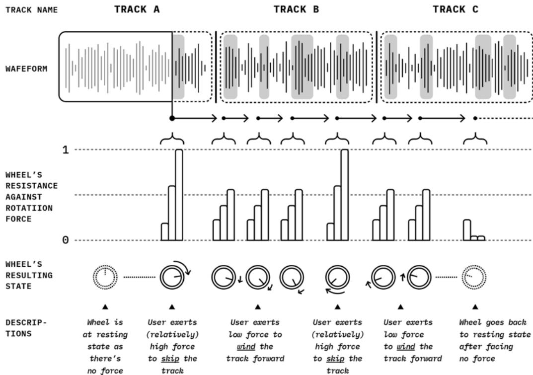
**Two-axis wheel.** In spite of being able to progressively venture to a further-distanced music piece by changing the direction/distance with every skipped piece of music, the means to do so with step-by-step basis until reaching a satisfactory distance is neither efficient nor intuitive. For this reason, being able to change tolerances of distance would be an effective tool do alleviate this issue.
