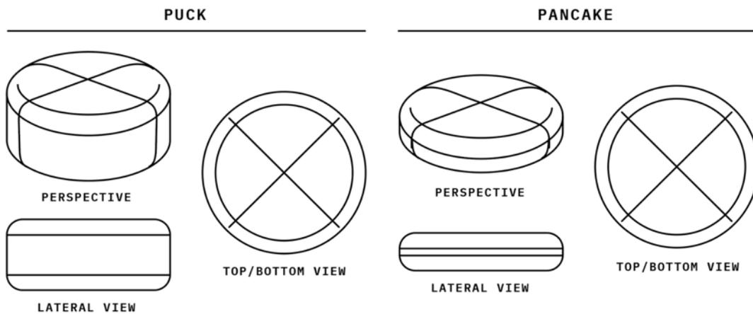
Figure 6.24 - Perspective, lateral, and top/bottom views of puck-shaped and pancake-shaped filleted cylindrical slabs.
