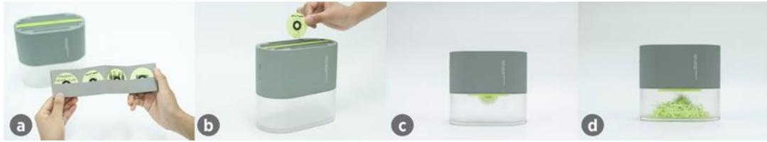
Figure 2.16 - muRedder's use scenario: user selects a song from their catalogue (a), inserts it (b) to the device, the music sheet gets shredded (c) as the music is played, its container (d) visualises the music listened in the past with a pile of shreds (Kim et al., 2019).
