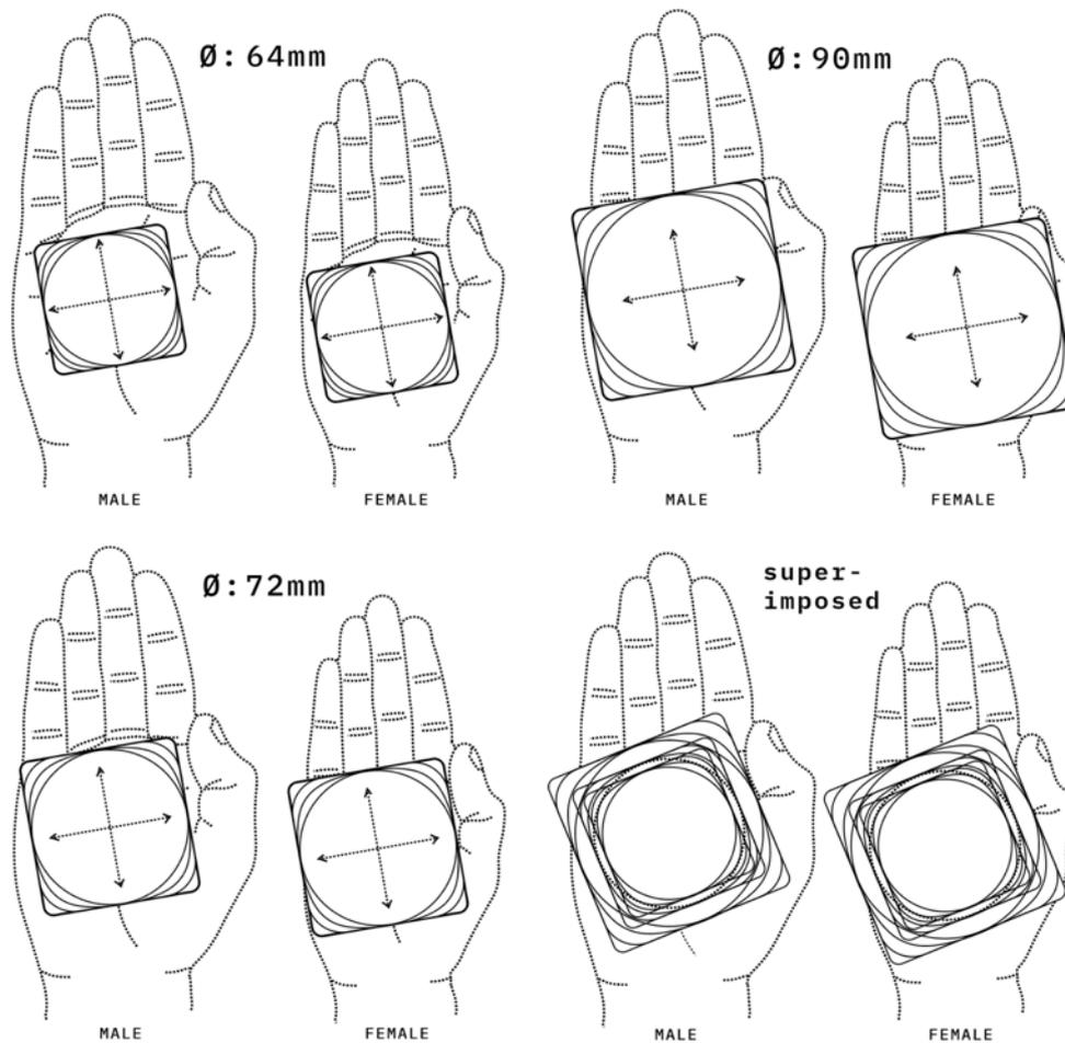
Figure 6.22 - A diagram visualising how primitive shapes between circle and square with diameters of 64, 72, and 90 millimetres compare to each other.
