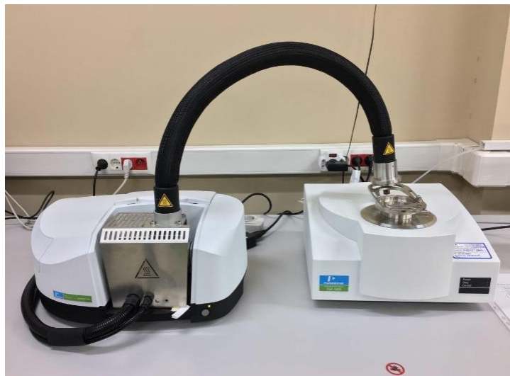
Figure 3.3 TGA coupled with an FTIR spectrometer at the Composite Material Characterisation Laboratory at Center for Wind Energy Research, Middle East Technical University [48].
