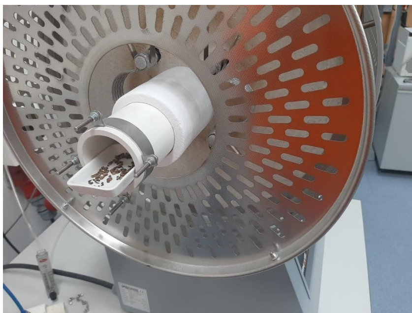
Figure 3.7 Olive residue particles put into the horizontal furnace for slow pyrolysis experiment
