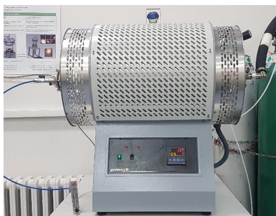
Figure 3.4 Horizontal furnace used for torrefaction and slow pyrolysis experiments
