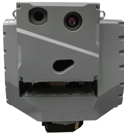
Figure 5.1: The 2 axes gimbal platform to be used in target tracking application (Photo Courtesy of ASELSAN Inc.).
