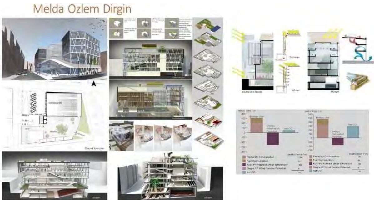
Figure 4. The designed Architecture department project incorporate the use of; natural light, natural ventilation with wind catchers, sustainable materials (constructed out of wood and steel), double skin façade, shading elements, green roofs, collecting rain water, reuse of grey water, and solar panels. The proposed design had %32 reduction in annual energy consumption
