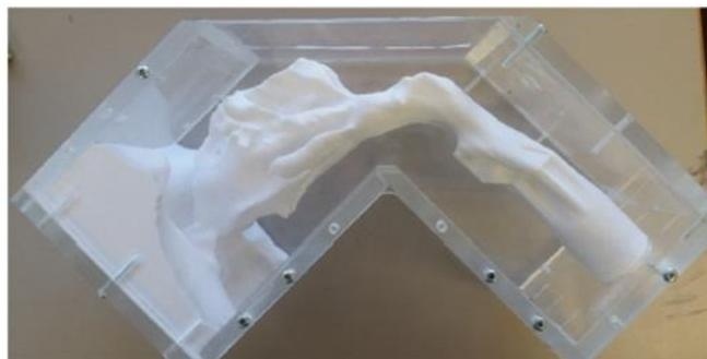
Figure 2.7: Casting box for PDMS with male mold [36]
