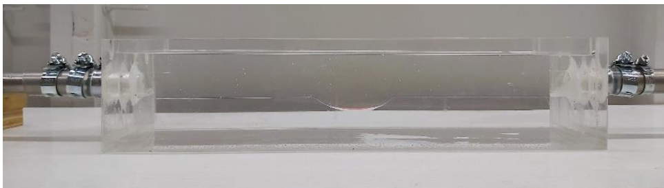
Figure 3.3: Working fluid filled in the vessel, and between the phantom and box to show RI match
