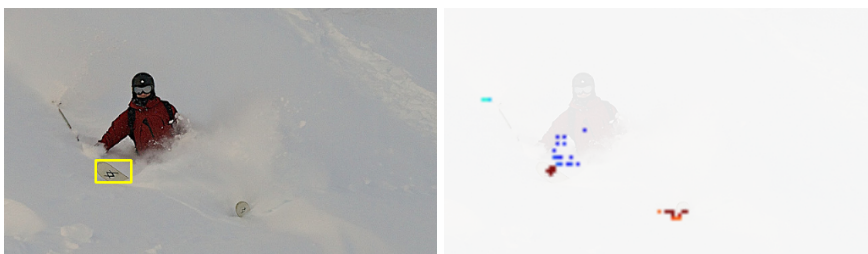
Figure C.3: Ski detection gets strong votes from other ski, ski baton and person .
