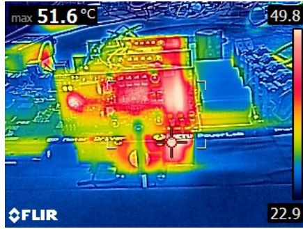
(a) Temperature Distribution on the Five-Phase Inverter, at t = 5 min.
