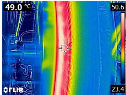
(a) Temperature distribution in the motor windings at t = 20 min.
