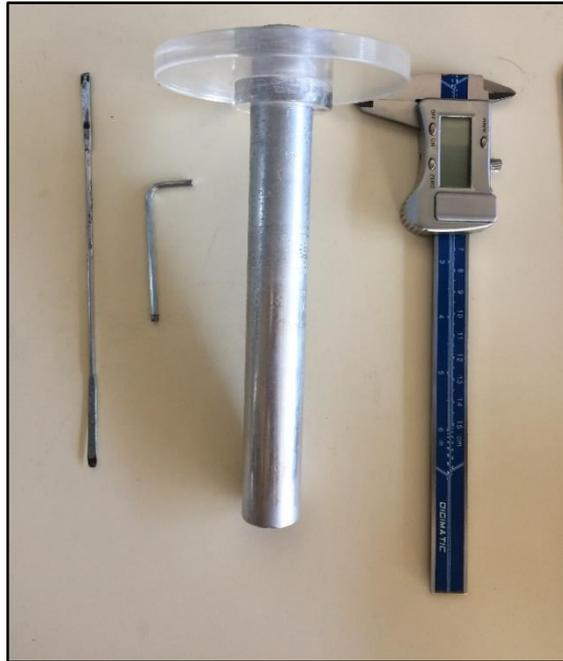
Figure 3.8. Tamping rod and caliper
