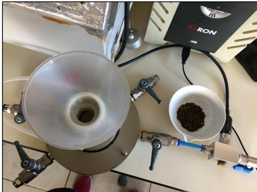
Figure 3.11. Measured mass and funnel
