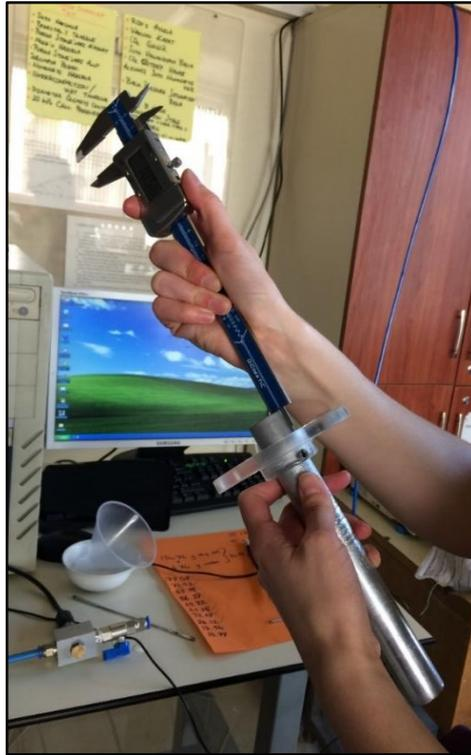
Figure 3.9. Height adjustment of the tamping rod
