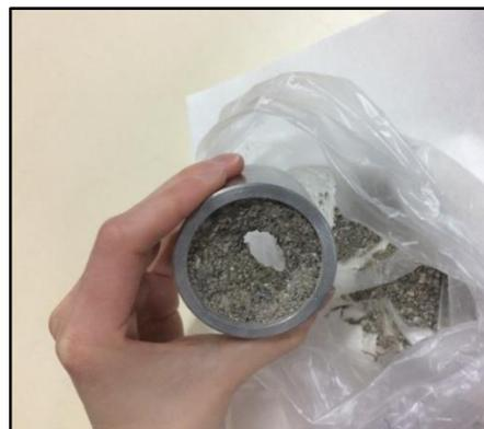
Figure 3.33. Removing specimen from the mold
