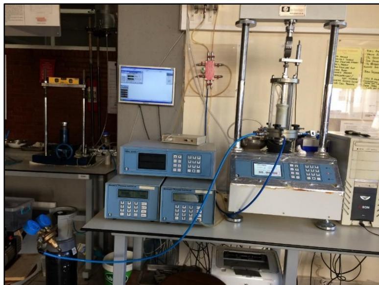
Figure 3.5. VJ TECH triaxial testing system
