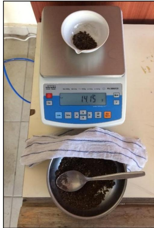
Figure 3.10. Mass measurement for a layer
