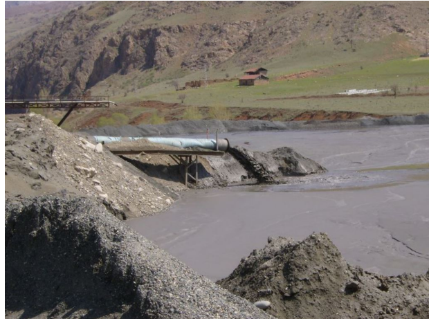
Figure 2. Discharge of the tailings to waste pool [20].
