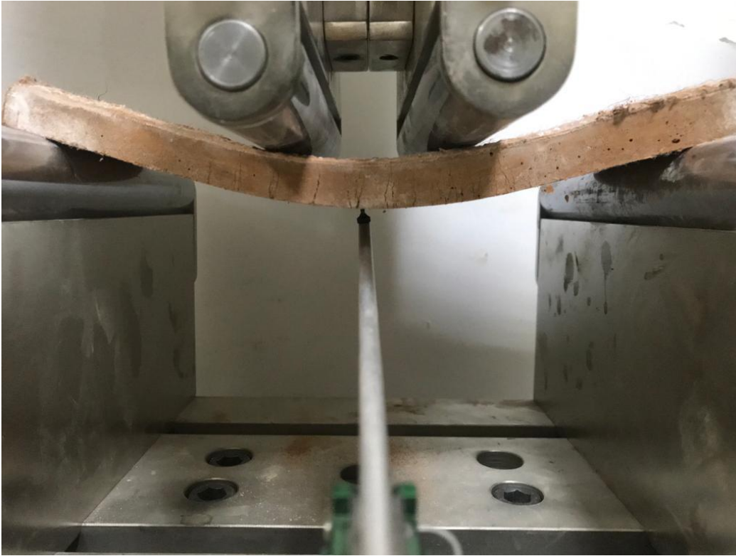
Figure 3.14. Midpoint displacement recording with deflectometer
