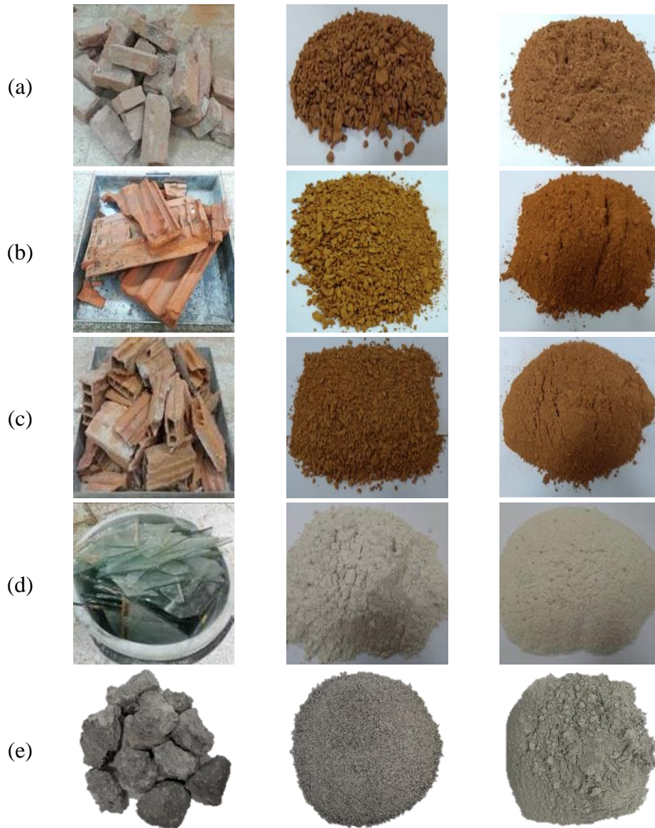
Figure 3.1. CDW-based materials in bulk, crushed and ground form red clay brick (a), roof tile (b), hollow brick (c), glass waste (d), concrete waste (e)
