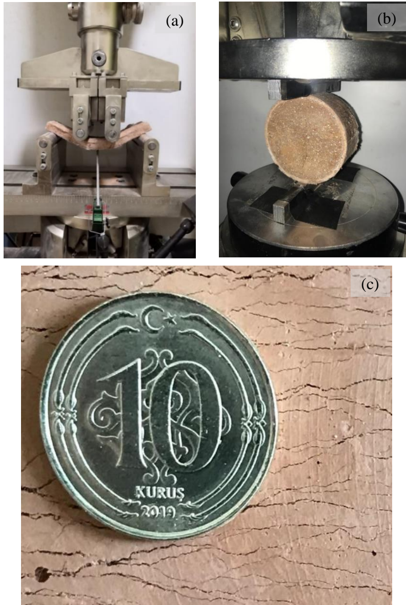
Figure 3.11. Preloading of (a) prismatic- and (b) disc specimens, and (c) cracks formed after preloading
