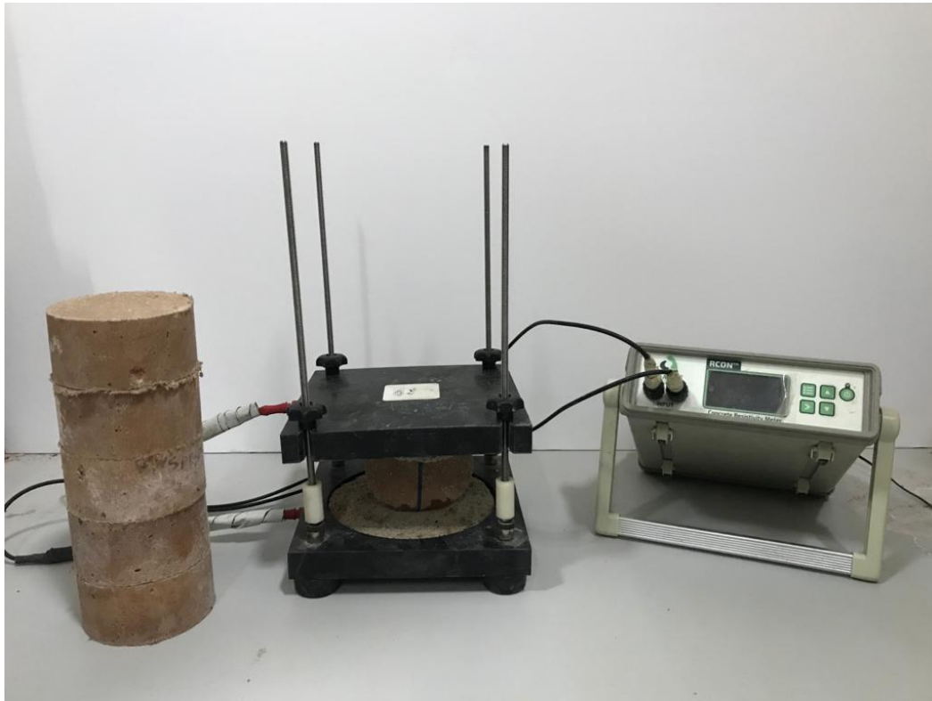
Figure 3.12. Electrical impedance testing device
