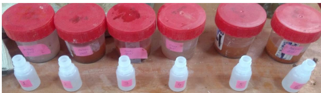
Figure 3.9. Preparing ICP-OES specimens
