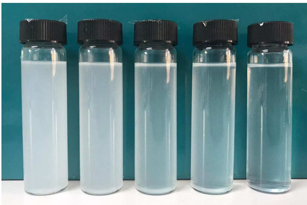
Figure 3.3.1.4 Turbidity variations of the solutions prepared by adding from left to right 0.22, 0.18, 0.11, 0.066, and 0.022wt.% Pluronic L61.
