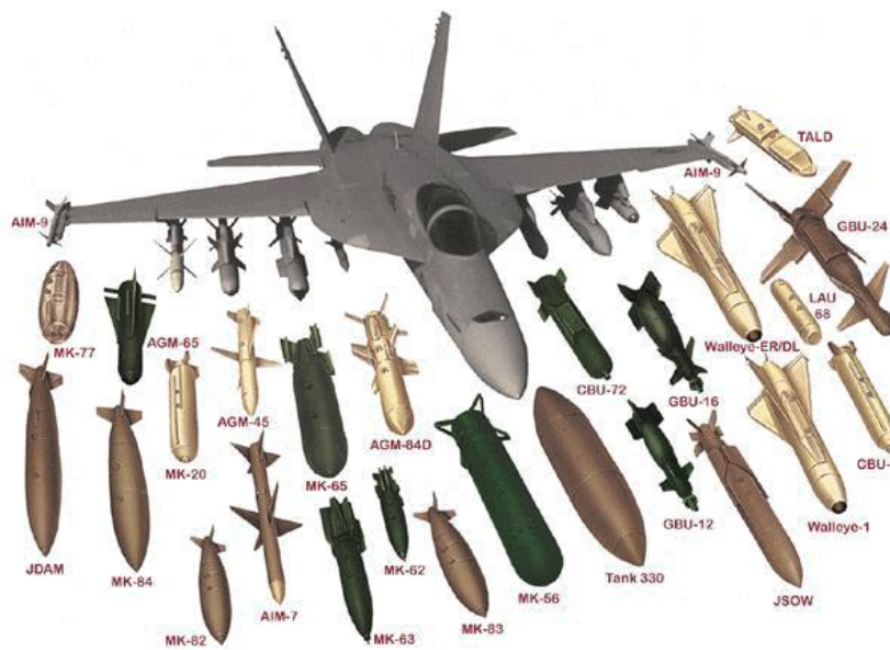
Figure 5.1 Modern Fighter Aircraft and Its External Store Inventory [55]
