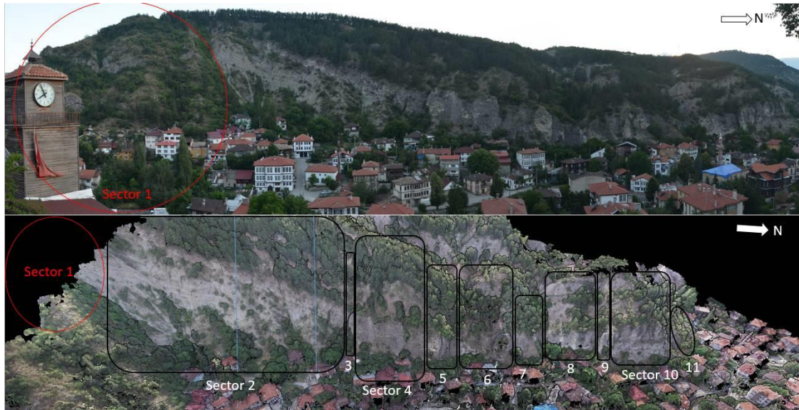
Figure 4. Geomechanical sectors defined as a result of a detailed evaluation of the rock mass characteristics
