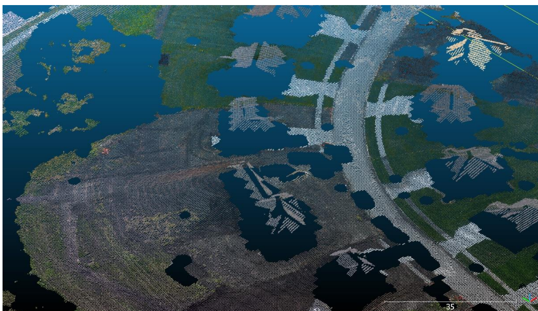
Figure 61: Eliminating vertical planes in Ankeny dataset using grid-based planarity values
