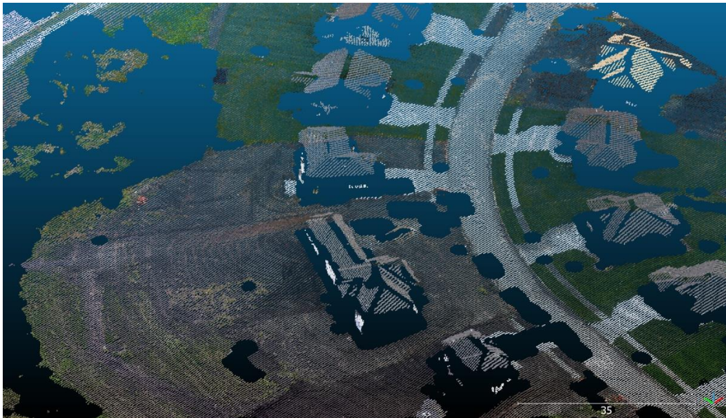
Figure 60: Ankeny dataset after approximate coplanarity filter is applied
