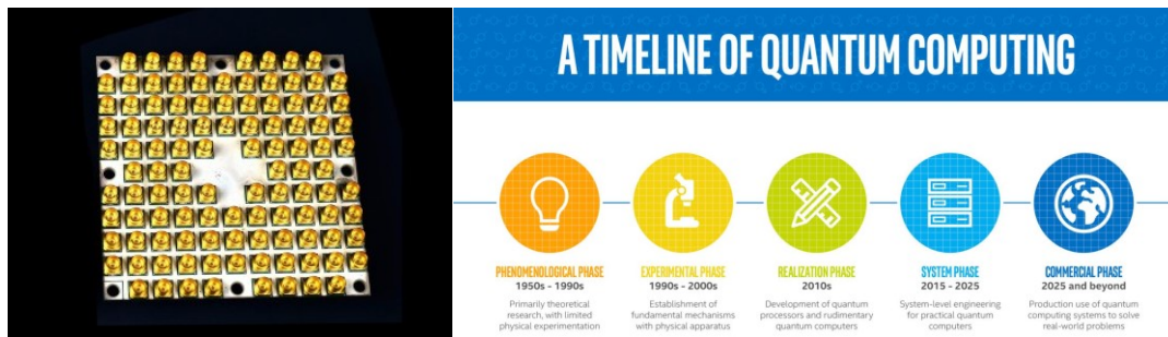
Figure 5.3. The Tangle Lake 49-qubit quantum processor (Intel, 2019) (left); A Timeline of Quantum Computing (IBM, 2018, 2020) (right)
