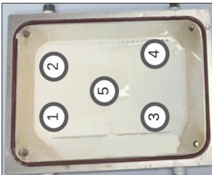
Figure 3.10. Scan points of degraded membrane
