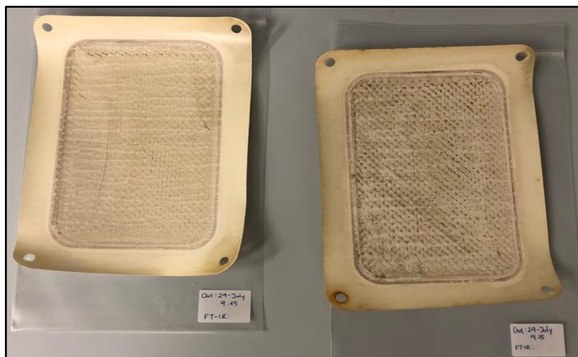
Figure 4.14. Rejuvenated membranes after drying 24 h
