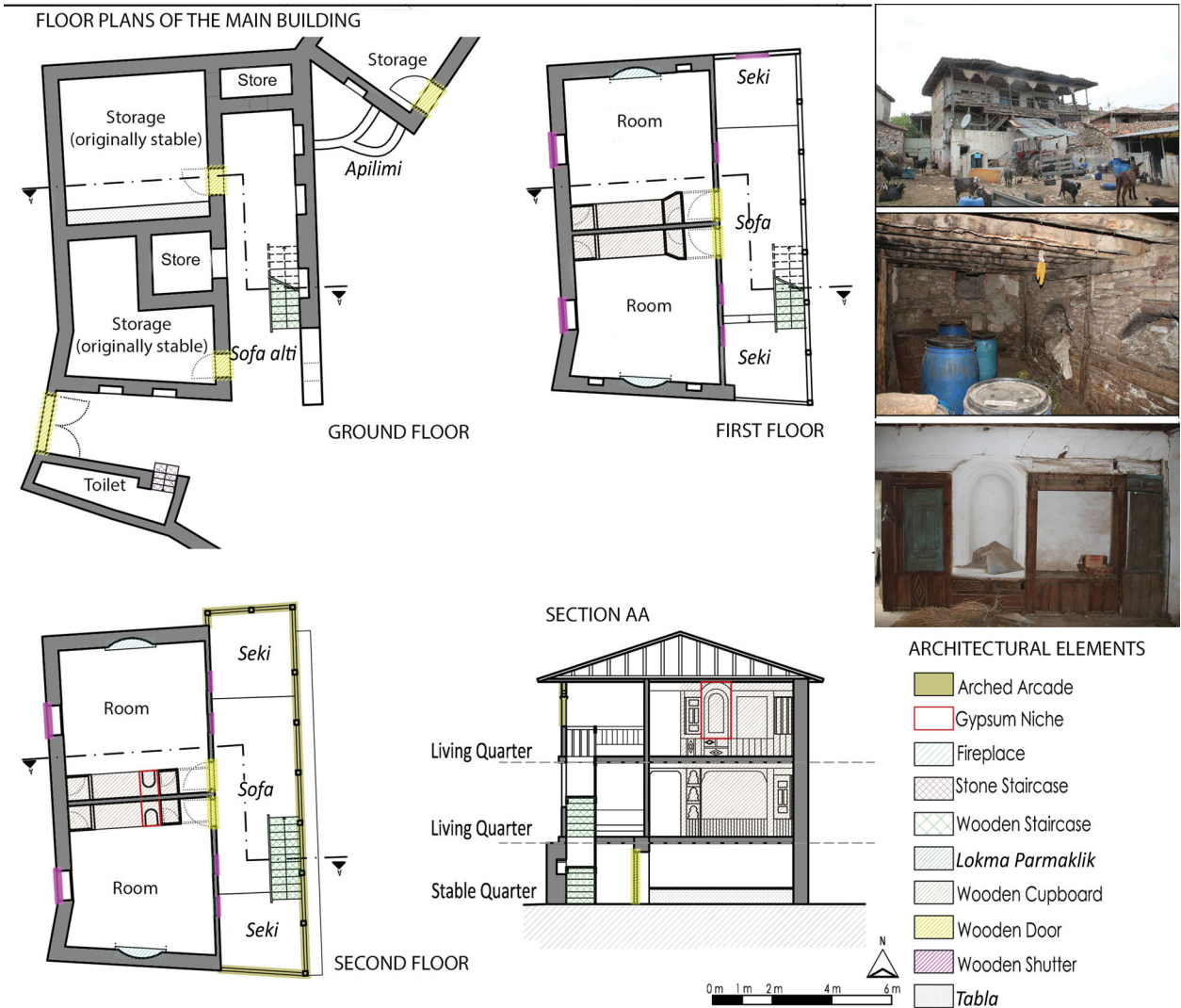
Figure 14. Reconstructed drawing of DB's house, which had a plan type that included an outer sofa (indicated as P1 in Fig. 9).
