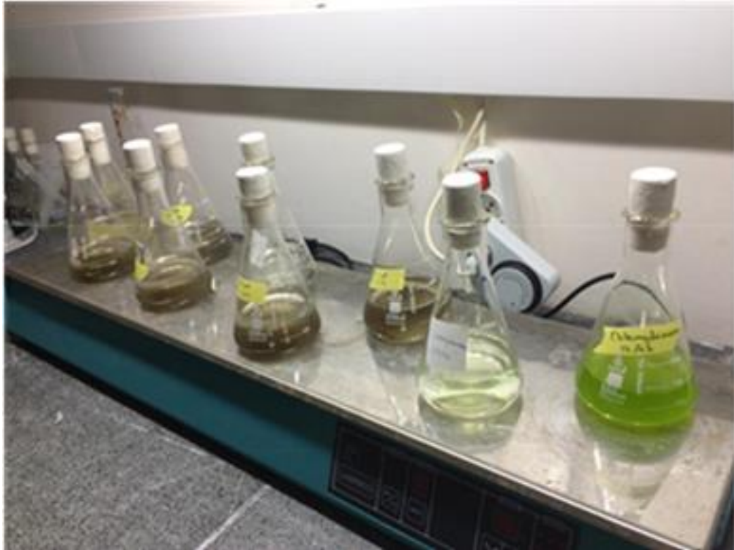
Figure 3: Phytoplankton culture set-up under a 60 \mu\text{m photon m}^{-2} \text{s}^{-1} light intensity, 14:10 hour L:D cycle, and at 22 \pm 1 \text{ }^\circ\text{C} .
