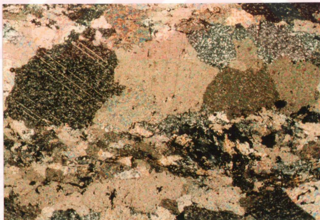
Figure 5 Photomicrograph of marble, foliated, containing graphite along planes of foliation (sample no. R-21, crossed nicols x40).
