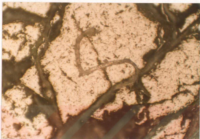
Figure 44. Photomicrograph of chromite showing nodular texture (sample no. C-6, crossed nicols).
