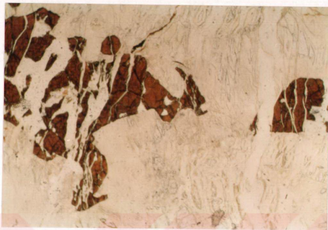
Figure 9. Photomicrograph of chromian spinel (picotite) in serpentized harzburgite; the grains show cataclastic texture (samp. no. R-26, plane light x 40).
