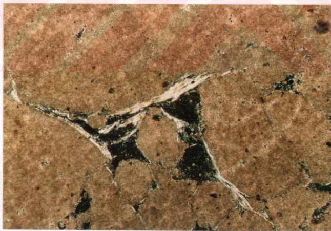
Figure 35. Photomicrograph of fine grained magnesite containing talc developed along fractures (sample no. M-4, crossed nicols x40).
