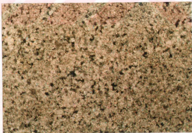
Figure 19. Photomicrograph of fine grained limestone (sample no. R-1, crossed nicols x40).
