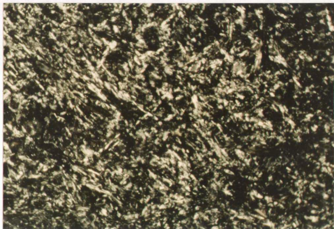
Figure 12. Photomicrograph of fine grained serpentinite with no traces of primary minerals (samp. no. R-19, crossed nicols x 40).
