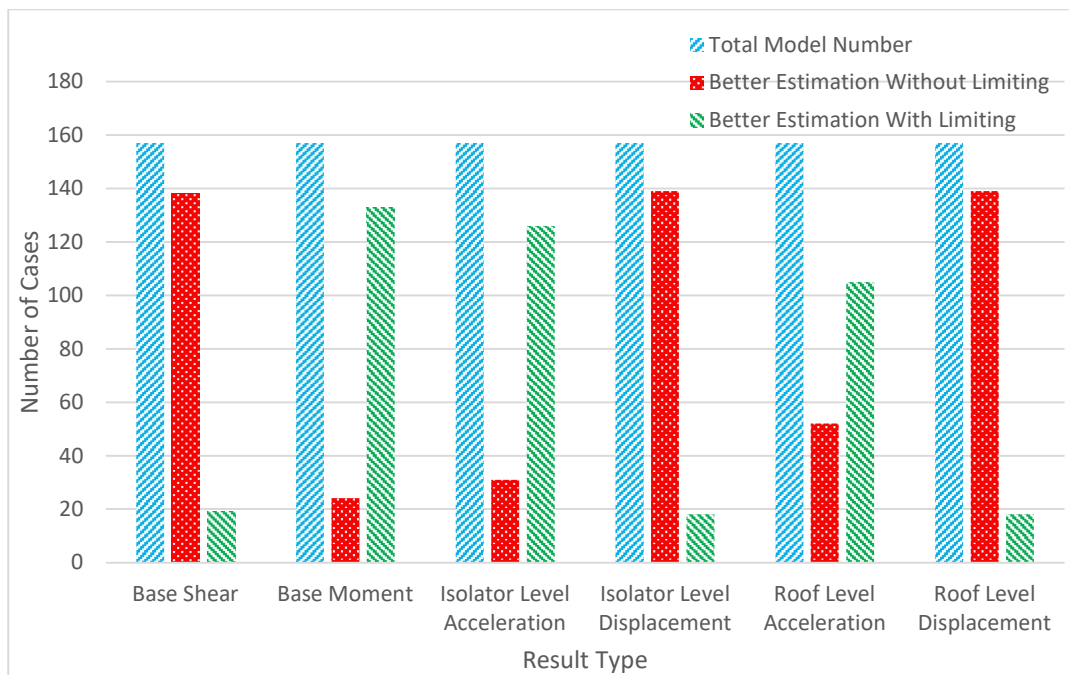
Figure 5.7. Number of Cases With Better Estimated Results According to The Limitation of The Equivalent Linear Damping Coefficient
