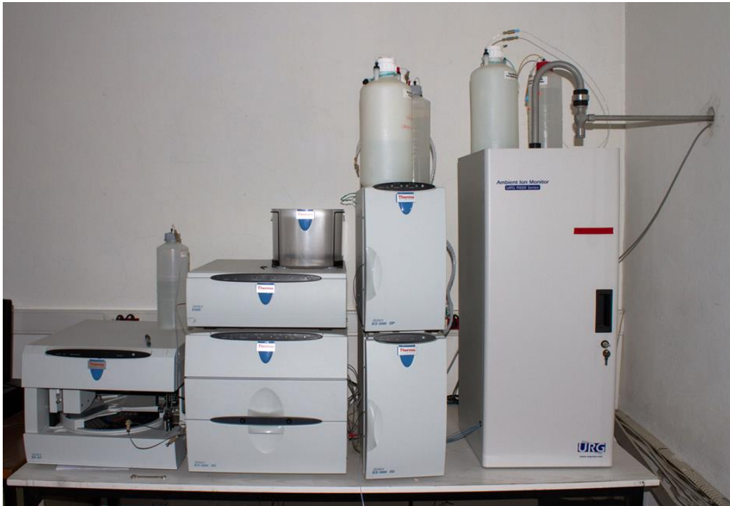
Figure 2.4 Ambient Ion Monitor Ion Chromatography (the sample analysis unit: ICS-5000, Thermo-Dionex, the sampling unit for the simultaneous collecting of PM 2.5 and their precursor gases: AIM 9000D, URG Corp., Chapel Hill, NC)
