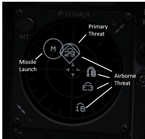
Figure 1: An example Radar Warning Receiver screen
