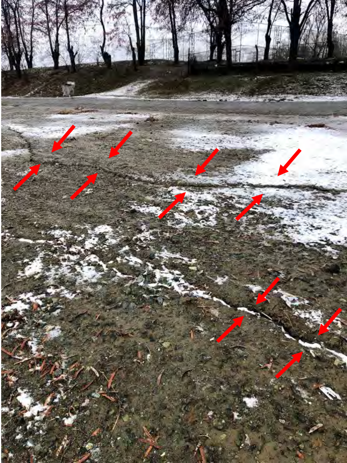
Figure 4.16. Seismically-induced lateral spreading ground deformations mapped on the beach of Hazar Lake ( 38^{\circ}26'50.7''N 39^{\circ}18'56.7''E / 31.01.2020 / 12:28)
