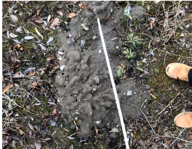
Figure 4.127. Surface manifestations of soil liquefaction in Hazar Lake (8 th stop)
