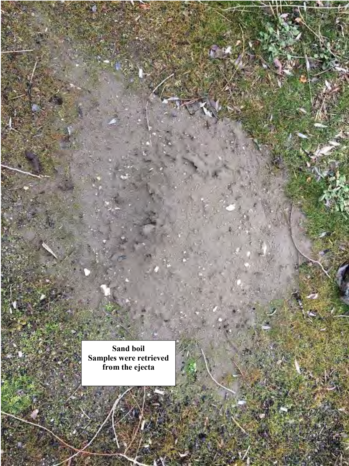
Figure 4.38. Sand boil observed in Stop 8 ( 38^{\circ}27'50.1''N 39^{\circ}24'01.3''E / 31.01.2020 / 14:43)
