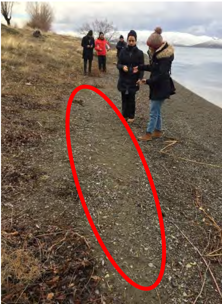
Figure 4.127. Surface manifestations of soil liquefaction in Hazar Lake (8 th stop)
