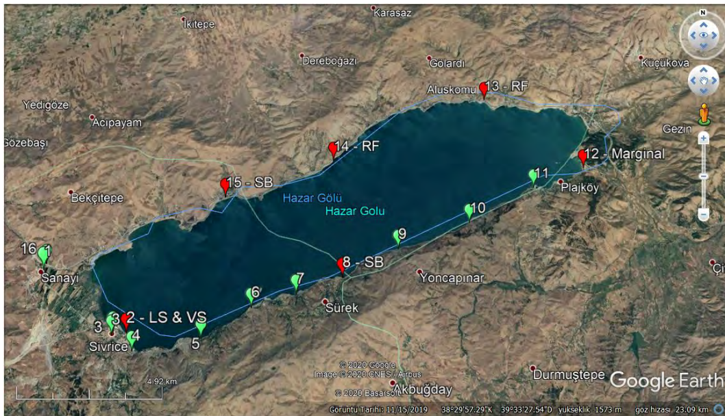
Figure 4.121. A summary of ground failure observations along the shores of Hazar Lake (Green pins indicate Non-Liquefied sites, Red pins indicate sites with surface deformations, RF: Rock fall, LS: Lateral spread, VS: Volumetric settlement, SB: Sand Boil)
