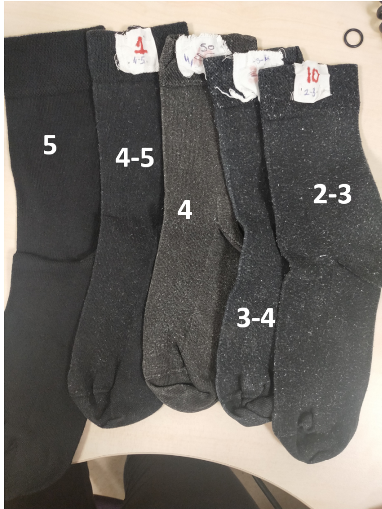
Figure 1.3: Sock example with different amounts of the piling on the surface. We received this example from the Arcelik team as a reference at the beginning of the study.
