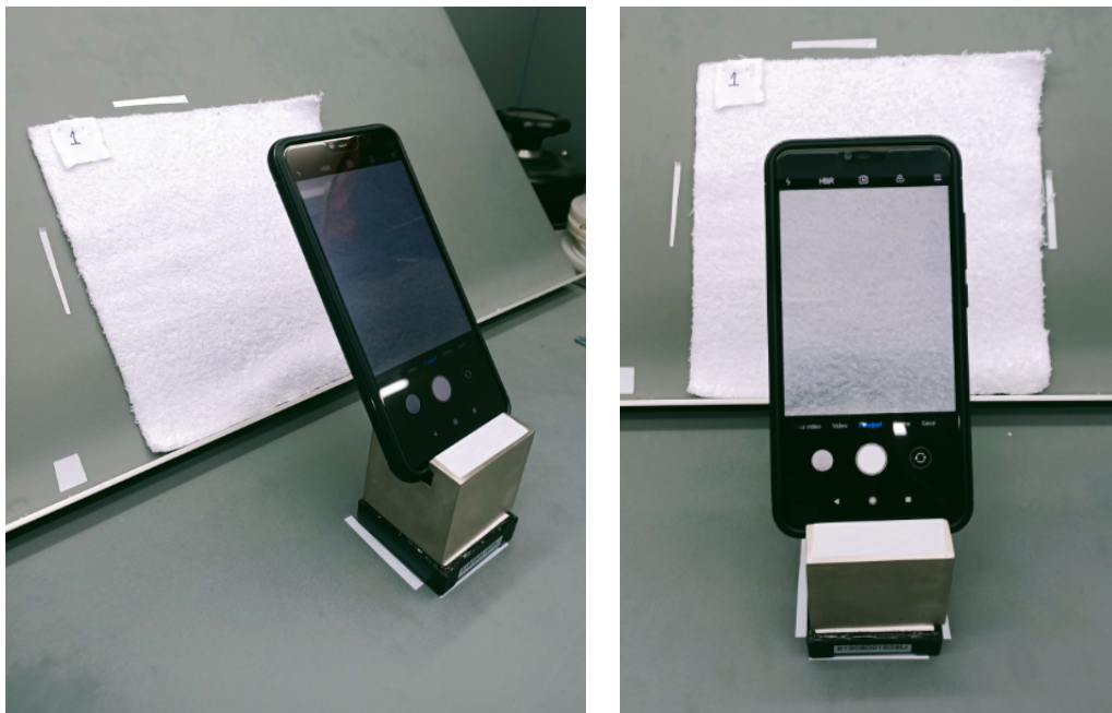
Figure 4.3: The final setup to capture sample images that are ready to use in softness analysis.
