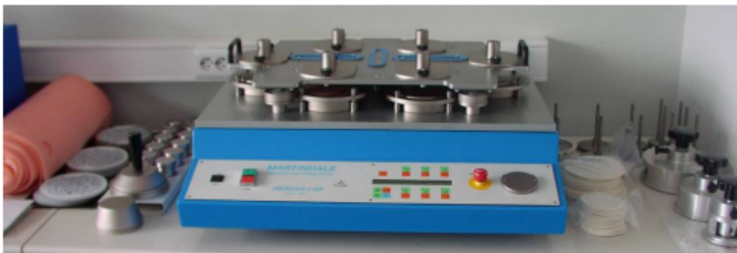
Figure 2.3: The Martindale Abrasion and Pilling tester machine. The machine has movable small discs on different sizes which are also optimizable in size and characteristics. Figure taken from [38].
