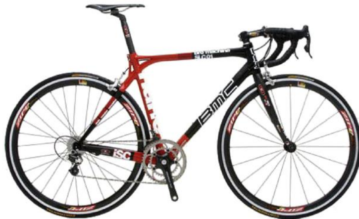
Figure 1.9: Bicycle whose framework is made of CNTRC [11].
