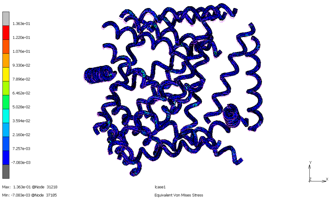
Figure 4.30: Equivalent Von Mises stress distribution on interface (5 revolutions, (6,6), randomly oriented case).
