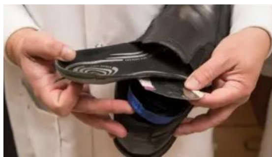
Figure 2.18: A thin sensor made of CNTRC placed inside a shoe to measure foot pressure [43].
