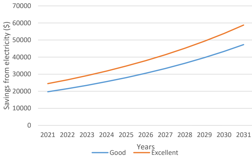
Figure 5.8. Annual change in savings from electricity for 15-storey building for a household for 10 years with respect to non-green building
